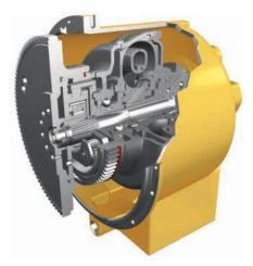
**Torque Divider**. A single-stage torque divider sends 70 percent of engine torque through a converter and 30 percent through a direct drive shaft for greater driveline efficiency and higher torque multiplication.
