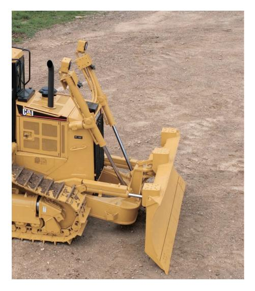
**Cat**<sup>®</sup> **Blades**. All blades feature a strong box-section design that resists twisting and cracking. Blades are made of Cat DH- $2^{TM}$  steel that has high tensile strength and stands up to the most severe applications. Heavy moldboard construction and hardened bolt-on cutting edges and end bits add strength and durability.
