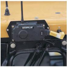
**Product Link.** The optional Product Link system is a factory installed or easily retrofitted wireless system that simplifies equipment fleet tracking. Using satellite or cellular technology, the system automatically reports key machine parameters such as location, machine hours, active and logged service codes and security alarms. Depending on the Product Link version, it can connect with other on-board systems, issue e-mail or pager alerts and provide fuel consumption data.
