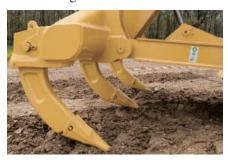
**Multi-Shank Ripper.** The multi-shank parallelogram ripper offers the choice of one, two or three shanks depending on job conditions. Curved or straight ripper shanks are available.
