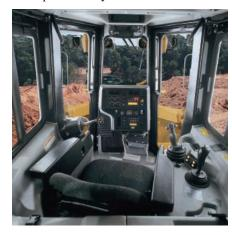
**Caterpillar Monitoring System.** The D6R III features a flexible monitoring system that is easily upgraded by flashing software. As technology changes and new electronics and software become available, this upgradable monitoring system allows the machine to be easily updated and take advantage of improvements.
