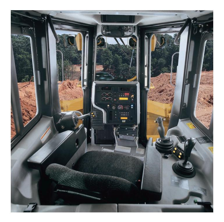
**Cab.** An isolation-mounted, pressurized cab reduces noise and vibration for operator comfort. The cab is pre-wired for a 12-volt or 24-volt radio, equipped with two speakers, an antenna and a radio mount recessed in the headliner.
