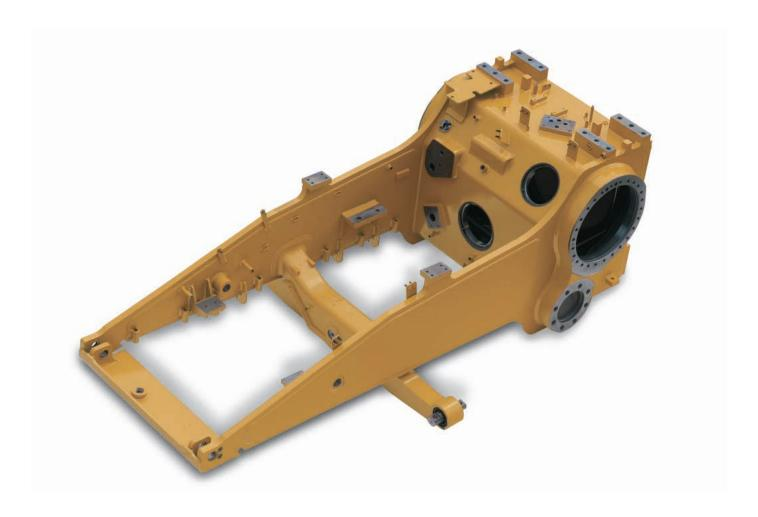
**Frame and Castings.** The D6R III frame is built to absorb high impact shock loads and twisting forces. The frame has a reinforced saddle and a welded front cross-member that add strength to the frame to better handle lateral and twisting forces. Steel castings augment the strength of the main case.
