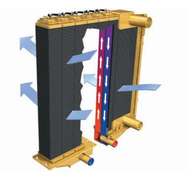
Advanced Modular Cooling System (AMOCS). Using a two pass system, the AMOCS radiator provides more efficient heat exchange and improved cooling capacity over the D6R Series II. The coolant is routed from a sectioned bottom tank up the front side, over the top of the core and down the engine side of the core to the bottom tank. This flow pattern allows the coolant to pass through the radiator twice for better cooling.
