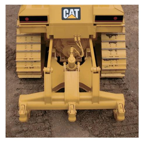
**Winch**. A single lever control actuates both clutch and brake functions to improve operator efficiency.
